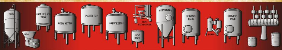
In the first step of brewing, some of the Barley Malt in our silo is coarsely ground in our grist mill. It's then mixed with warm water from the Hot Liquor Tank in the Brew Kettle and allowed to sit for about an hour. **During this "mashing"** process, enzymes in the malt break down barley starches to simpler sugars, resulting in a very sweet liquid called "wort", (pronounced wert).
